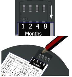
**3.** Switch all four DIP switches to the **`ON**' position using a pen or pencil
