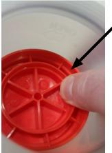
**3.** Begin pumping the grease into the Cup, as you begin use your thumb and depress the one side of the Red Cartridge to release any air pockets.
