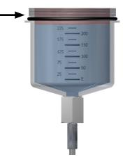
**4.** Fill the cup up with grease until the Red Cartridge is level and flush with the rim of the Cup. Ensure there are no air pockets. If you can visually see an air pocket, remove the adapter fitting and depress the Red Cartridge by hand to push the grease out. Restart from step 2 again
