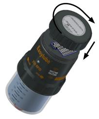
**7.** Put the battery back into the Lubricator and screw the Drive unit top Cap back on securely. The LED indicator light will auto blink for 5 seconds to initiate. When the LED indicator light goes off, it indicates that the Lubricator is now in operation mode with no alarms.
