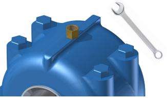
**2.** Use the correctly selected direct mount adapter fitting and screw it into the plumber block. Do not over tighten as you may risk breaking the fitting or damaging the thread on either the fitting or Plumber Block
