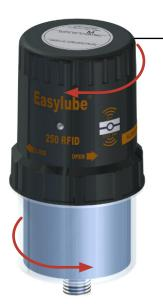
**4.** Screw the Prefilled Grease Cup into the Lubricator Drive body and ensure the Press Plate makes contact with the Red Piston on the Cup. A small amount of grease should discharge from the Cup which indicates that the Press Plate is pressing against the Red Piston.
