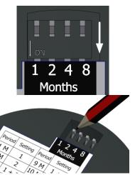
**6.** You can now set your lubricator to the desired month setting, refer to the table on top of the lubricator which indicates which DIP switches need to be switched to the **`ON**' position for all 12 month options
