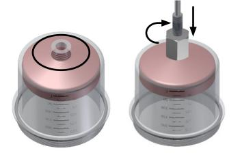
**2.** Locate the 1/2" Male thread on the cup & screw on the adapter fitting and attach the hand operated grease gun
