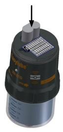
**4.** Insert the battery to initiate the Lubricator; during **TEST** mode, the Lubricator will automatically rotate and push the Red Cartridge in the Cup every 7 to 8 seconds, a small amount of grease should start to discharge
